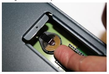
**Caution:** DO NOT USE A METAL OBJECT TO PRY OUT THE BATTERY SINCE IT MAY SHORT THE BATTERY AND DAMAGE THE BATTERY HOUSING.
